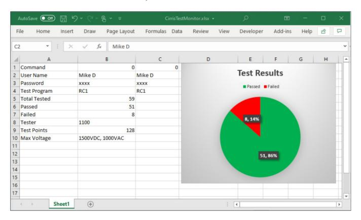
In this case, Excel is installed on a network station with OPC UA client software, which monitors a Cirris OPC UA Server and updates Excel. Real-time test information can be simultaneously transmitted from one or multiple Easy-Wire stations that have OPC UA Server enabled. The OPC UA communication standard presents a positive framework for future plant floor automation and process communication.
